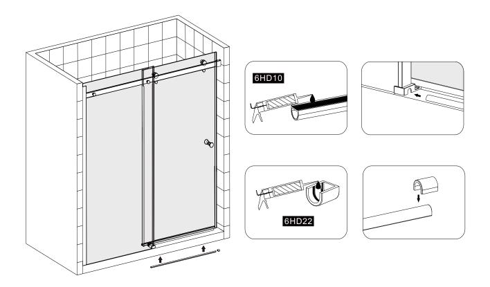
Finally, at all points connected to the wall, the bathtub and the profiles, use silicone sealant only on the outside of the shower enclosure. Please do not take shower within 24 hours after silicon sealant.
