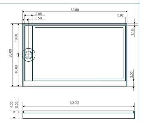
Shower base does not have a molded tile flange. 3 fiberglass tile flanges are included and must be installed with 100% silicone and screws used on the side of the base after the installation position of the base is established.
