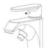
Step.3 Take out the handle and remove the brass escutcheon
