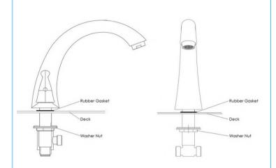
**2.** Unscrew the washer nut and place the rubber gasket and spout above the deck. After, secure the washer nut from underneath the deck.
