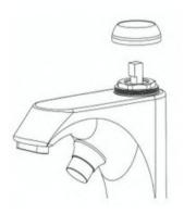
Step.5 Remove the cartridge and replace it with new piece.
