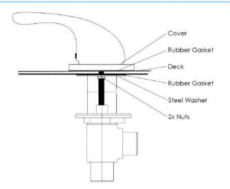
Unscrew the 2 nuts securing the steel washer and rubber gasket. In this order, remove the steel washer and rubber gasket, place your lever on the deck, replace the rubber gasket and the steel washer. Firmly secure the 2 nuts to hold the fixture in place.
