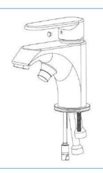
Step.2 Use an Allen wrench to remove the handle Screw.
