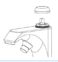
Step.5 Remove the cartridge and replace it with new piece.
